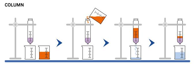
Prepare a column packed with scavenger silica and remove heavy metals by flowing down a solution containing heavy metals.
