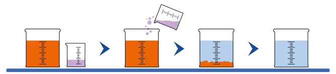
Heavy metals can be removed by adding scavenger silica to the solution containing heavy metals, stirring for a certain period of time and filtering.
