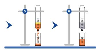
**Desorption solvent:** 2% thiourea / 1 M HCl / MeOH solution. 1 Set the column with Diamine Silica 2 Flow down the Pd solution 3 Wash the column with solvent 4 Add desorption solvent 5 Collect the eluted Pd 6 Complete elution and finish SH Silica has strong adsorption force with Pd and does not elute under these conditions.
